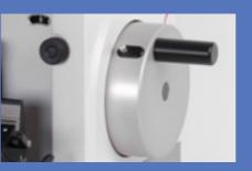
With the conveniently integrated locking lever on the hand wheel the rotation of the wheel can be locked at
